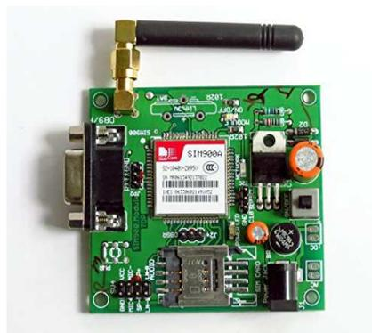
**Figure 6: GSM Module**
